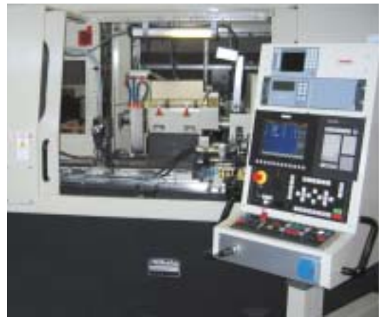
The grinding center chosen by Hanchuan Machine Tool is controlled by a Num Power 1050 CNC System.
